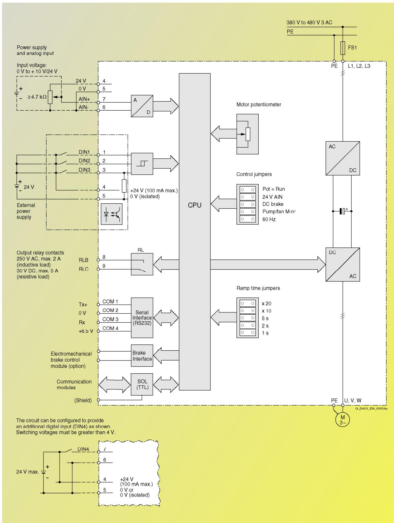
The circuit can be configured to provide an additional digital input (DIN4) as shown.
